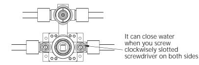
Note: If only close one side that it will cause faucet abnormal outlet water, for normal outlet water please make sure the adjusting position on both sides is open (counterclockwise to open).
