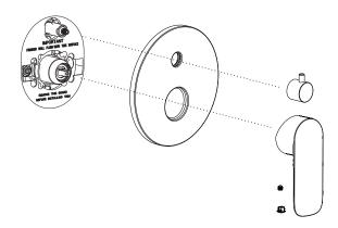
According to the figure below, please correctly adjust the direction of water separator handle.
